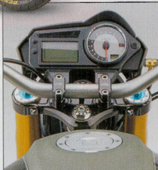
Project Brave Heart's headlight, mini-fairing and gauge cluster come from a $99. A custom triple clamp holds one-off bar risers.
